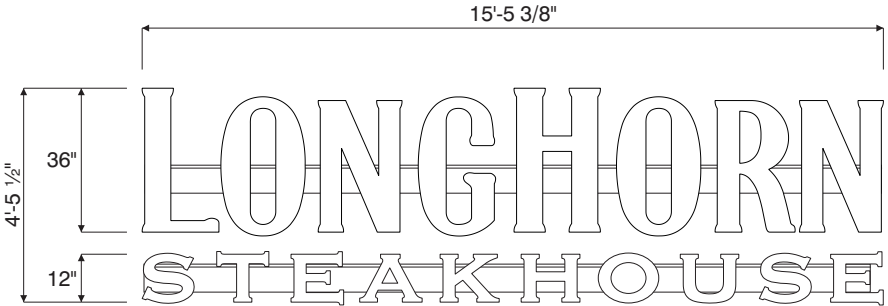
36" Channel Letters on Raceway (Internally Illuminated w/LED) Utilized Square Footage: 68.9 Scale: 1/4"=1'
